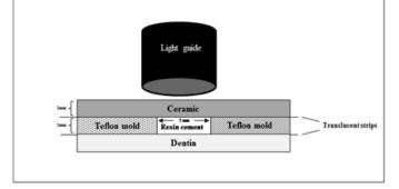
Figure 1. Schematic illustration of specimen preparation.
