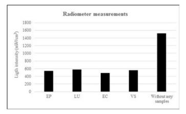
Figure 3. Radiometer measurements of polymerization light intensity (mW/cm2) through ceramic materials tested and without any samples. (EP: IPS e.max Press, LU: Lava Ultimate, EC: IPS e.max CAD, VS: Vita Suprinitiy).
