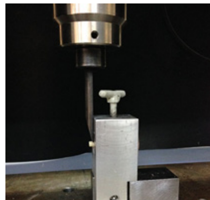
Figure 1: Shear bond strength test was applied to the tested samples.
