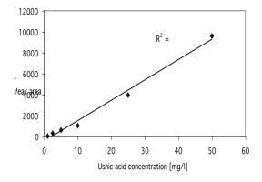
Figure 1: Standard calibration curve for the quantification of usnic acid by HPLC
