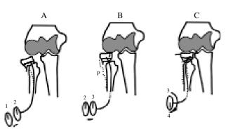
Fig. 2. Diagram demonstrating the reduction of the fracture by intramedullary pinning.
