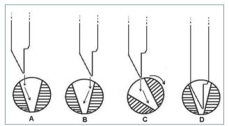
Fig. 5. The nail and distal interlocking screw (DSBLS) is drawn from the lateral aspect. The guiding effect is seen even if the nail drops anteriorly (A) or posteriorly (B) within a certain range. If the nail drops more anteriorly (C), the DSBLS is turned anteriorly and the nail is thusly caught by the DSBLS, and it returns to normal position by moving the nail further (D).
