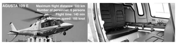
Figure 2. General outlook and technical characteristics of the ambulance helicopter used for transportation of patients with acute myocardial infarction for PCI
