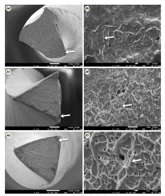
Fig. 1. SEM appearances of the HyFlex CM, Typhoon Cm and EdgeFile X3 files after cyclic fatigue testing. A-C-E: General view of EdgeFile X3 (a), HyFlex CM (c) and Typhoon CM (e) instrument B-D-F: High-magnification view EdgeFile X3 (b), HyFlex CM (d) and Typhoon CM (f) instrument showing fatigue striations typical of cyclic fatigue.
