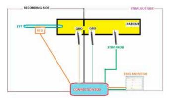
**Figure-1:** Schematic view of the monitoring system generated by recording and stimulation (EMG: Electromyography, ETT: Endotracheal tube, RE: Recording electrodes, GE: Grounding electrodes, SP: Stimulator probe)
