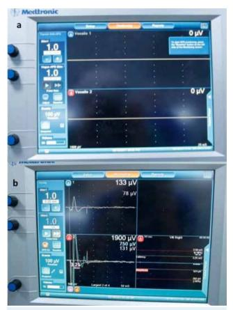
**Picture-3: a)** Two EMG channels opened at the monitor screen of Medtronic NIM-Response 3.0: 1 (blue) left vocal cord; 2 (red) right vocal cord. **b)** Two EMG channels that opened at the left when continuous vagus stimulation is performed with Medtronic NIM-Response 3.0 device, follow-up screen for continuous vagus stimulator probe opened for right vagus at the bottom right
