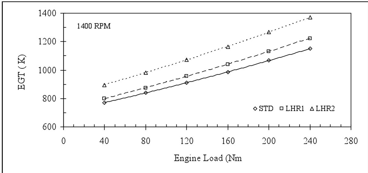
Figure 4. Comparison of EGT by engine load at 1400 rpm.
