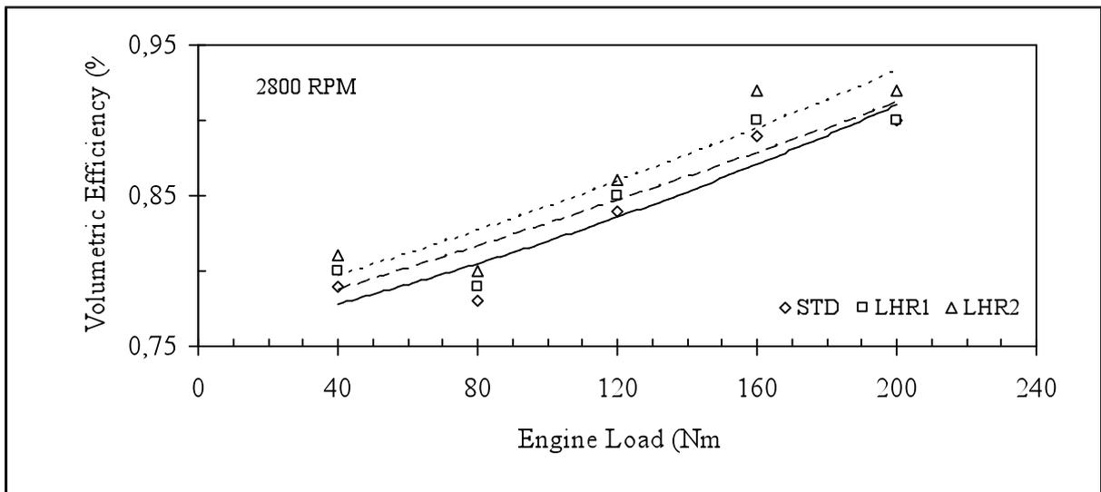
Figure 9. Comparison of volumetric efficiency by engine load at 2800 rpm.
