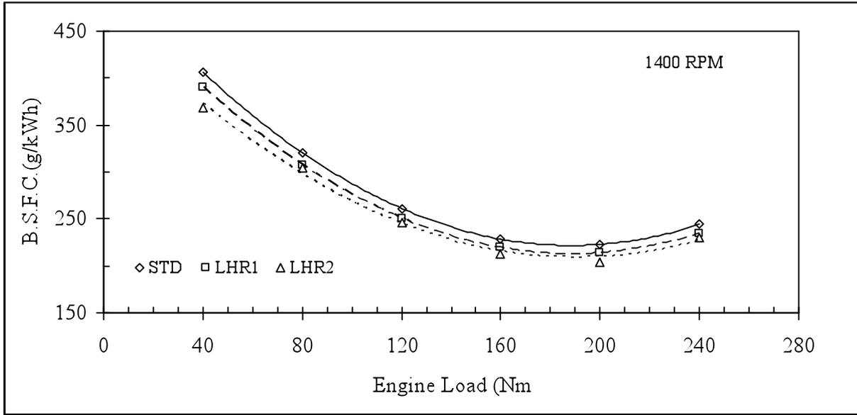
Figure 2. Comparison of BSFC by engine load at 1400 rpm.
