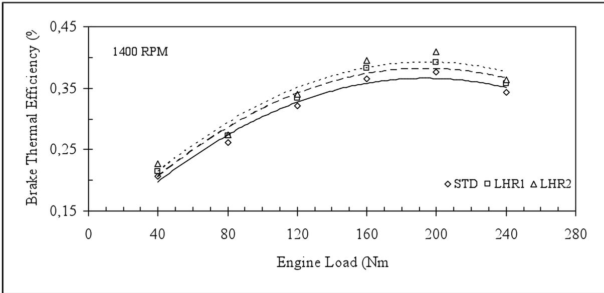
Figure 6. Comparison of brake thermal efficiency by engine load at 1400 rpm.
