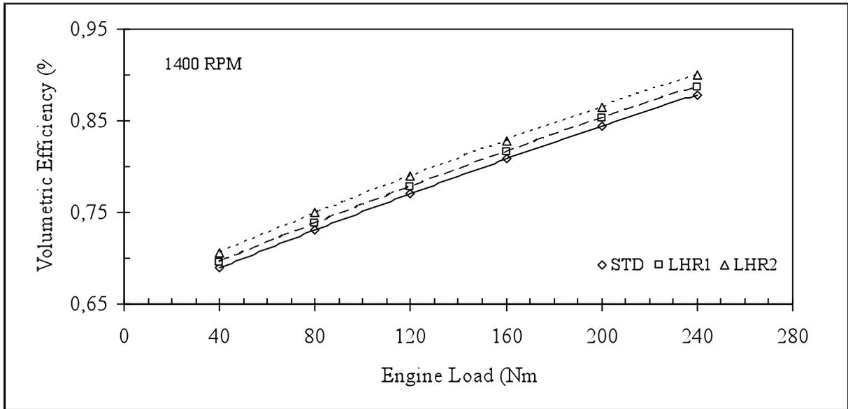
Figure 8. Comparison of volumetric efficiency by engine load at 1400 rpm.
