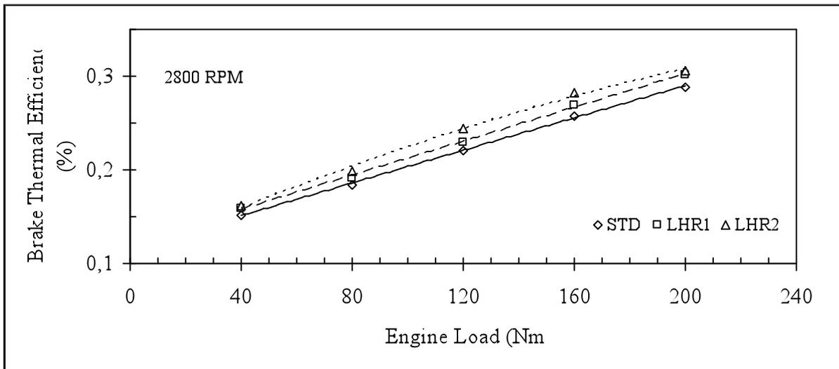
Figure 7. Comparison of brake thermal efficiency by engine load at 2800 rpm.
