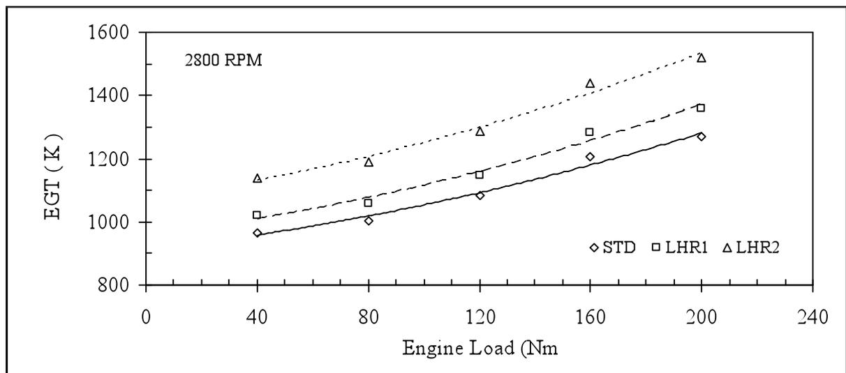
Figure 5. Comparison of EGT by engine load at 2800 rpm.
