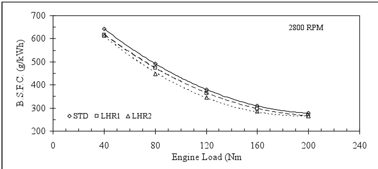
Figure 3. Comparison of BSFC by engine load at 2800 rpm.
