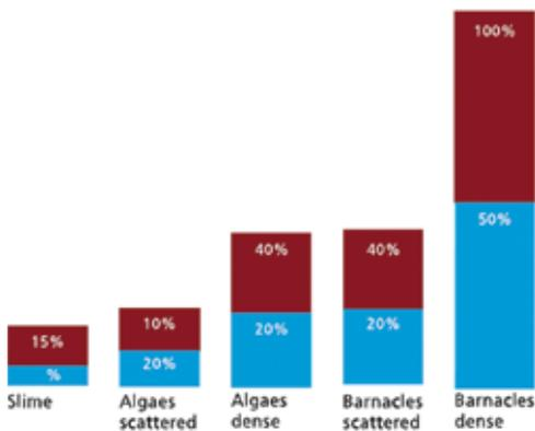
Figure 6 Fouling impact on fuel consumption (CleanHull, 2012)
