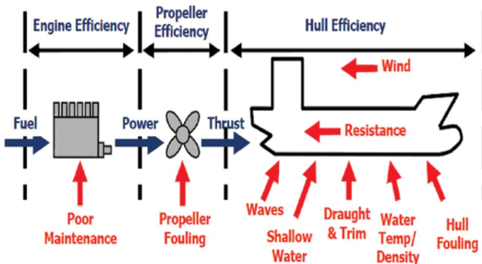
Figure 1 Variables influencing energy efficiency (Pedersen BP, 2009)
