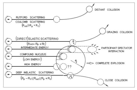
Figure 1: A sketch showing the wide spectrum of modes of interaction in charged particle encounters with a heavy nucleus. The energy of the projectiles along with the interaction radius seem to play an important role in identifying the reaction products formed in the exit channel and in determing the mode of interaction.
