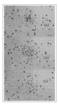
Figure 3: Photomicrographs (a, b and c) of three exceptionally high multiplicity events (or clusters) as observed in CR-39 exposed to 960 MeV/u- <sup>238</sup>U ions. The study of the characteristics of the etch pits comprising these events shows that most probably they were formed by some an isotropic source.
