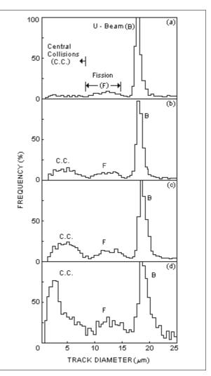
Figure 7: A set of four histograms showing diameter distributions of etch pits due to incident uranium beam (Peak 'B"), peripheral collisions resulting in fission fragments (humb 'F') and the particles formed in Central Collision (C.C.). It is quite apparent that the contribution of fission fragments and the light reaction products formed as a result of central collision go on increasing as the particle penetrates into the CR-39 stack.
