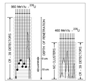
Figure 2: Stacks of CR-39 plastic track detectors exposed to <sup>238</sup>U-ions with energies of 460 MeV/u and 960 MeV/u at BEVALAC (Berkeley). Binary fission was found to be the most dominant mode of interaction at both the energies. Some (rare) three prong events were also observed. The exceptionally high multiplicity events (clusters) were observed only in the case of the stack exposed to 960 Mev/u- <sup>238</sup>U ions.
