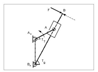
Figure 7: The wiper mechanism.
