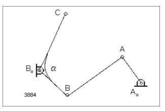
Figure 1: The four-bar linkage to be coordinated.
