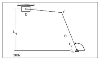
Figure 15: The slider-crank mechanism of the hack-saw.
