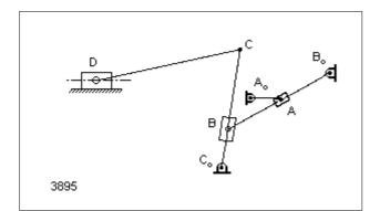
Figure 17: The resulting hack-saw.
