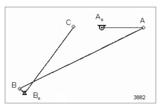
Figure 3: The resulting four-bar linkage.
