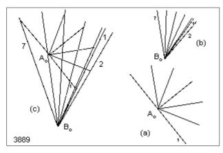
Figure 8: The procedure of synthesis for the wiper mechanism.
