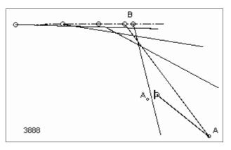
Figure 6: The resulting mechanism for the garage door, with the door at several locations.
