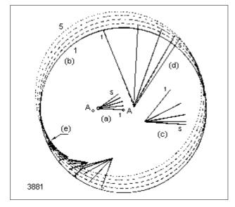
Figure 2: The procedure of synthesis for the four-bar linkage.
