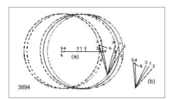
Figure 16: The procedure of synthesis for slider-crank mechanism of the hack-saw.
