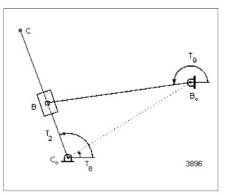
Figure 13: The secondFISC of the hack-saw.
