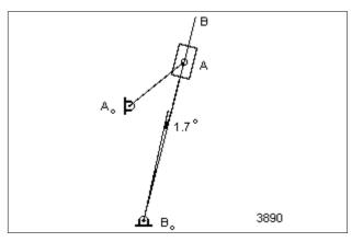
Figure 9: The resulting mechanism for the wiper mechanism.
