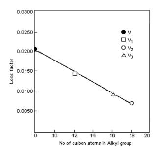
Figure 1: Loss factor versus number of carbon atoms for prepared alkyl phenol-formaldehyde disocyanate varnishes.
