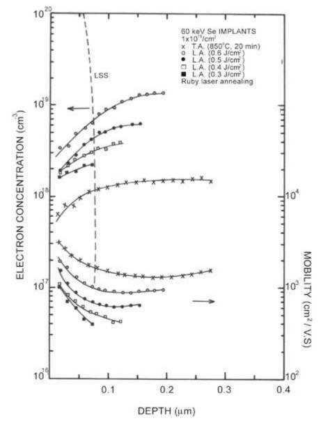
Figure 2: Depth profiles of the electron concentration and mobility measured on samples implanted with 60 keV Se ions at a dose of 1 x 10<sup>15</sup>/cm<sup>2</sup> and annealed Q-switched ruby laser at four different energy densities or thermally annealed.
