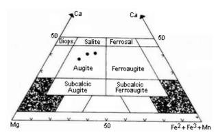
Figure 4: Classification of Pyroxenes from Egyptian Black Sands, as exhibited in the triangular diagram Ca-Mg-Fe atomic percentages.
