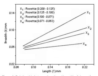
Figure 2: Relationship between length and breadth of zircons from Rosetta black sands. Lines are Reduced Major Axes (see text).
