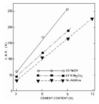
Figure 13: Relationship between the unconfined compressive strength and C.B.R. for Irbid soil-cement mixtures, stabilized with 0.0 N and 0.5 N of chemical additive, cured for 7 days.
