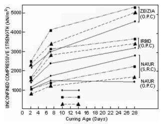
c) The effect of using chemical additives with the three soils stabilized by 12% cement content is shown in Figure 7. While the use of NaOH and  $Na_2CO_3$  with 0.5 normality was beneficial in case of the two soils from Zeizia and Irbid, it did not work with the greenish marly clay refered to as yellow Mediterranean soil from Na'ur.
