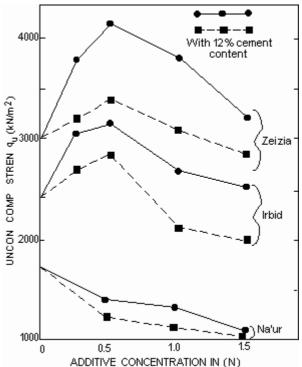
Figure 8. When the additive is beneficial, 0.5 N produce the optimum strength.
