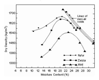
Figure 4: Moisture - Density relationship for all soils (standard Proctor T99-86).
