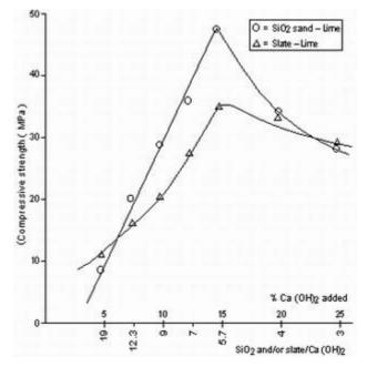
A maximum strength of 47.6 MPa is obtained after 4.5 hours autoclaving and 15%  $Ca(OH)_2$  content (silica sand/Ca(OH)\_2=5.67) while in our earlier investigation (1) the maximum strength of 25.8 MPa was recorded after 48 hours autoclaving at a steam pressure of 0.1 MPa (100°C) and 30.0% lime content.
