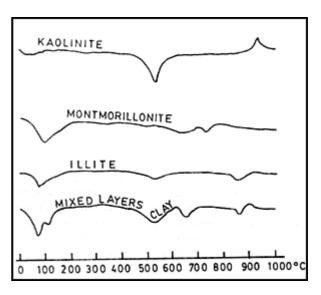
Figure 2: Thermograms of Typical Clays.
