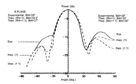
Figure 3: Radiation field patterns in E and H-planes of short backfire antenna.
