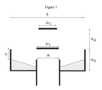
which varied from  $0.2\lambda$  up to  $0.6\lambda$  for the second small reflector, and the optimum value of  $0.4\lambda$  is displayed in measuring the radiation pattern of the antenna. The spacing between the back and first front reflector (d<sub>13</sub>) and between first and second front disks were provided with flexibility for optimum adjustment.
