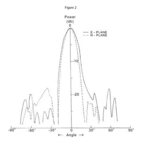
planes and that the highest values of the antenna under test gain is 17.2 db which is generally higher by 1.0 db where compared with the antenna of one small front circular disk, and about 6 db over the cup antenna (10), where the other parameters were shown in Table 2.
