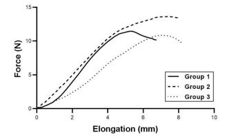
**Figure 3:** Elongation curves of tissues corresponding to tensile strength applied on groups according to mechanical tensile test graphics.
