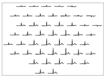
Figure 1. Example of 49 simultaneous non-contact MCG waveforms, arranged in a lattice on a plane covering an approximate circular area of diameter 21 cm
