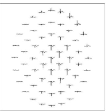
Figure 2. Example of 61 simultaneous non-contact MCG waveforms obtained by the Bochum magnetometer for one heartbeat for one subject MCG- magnetocardiogram
