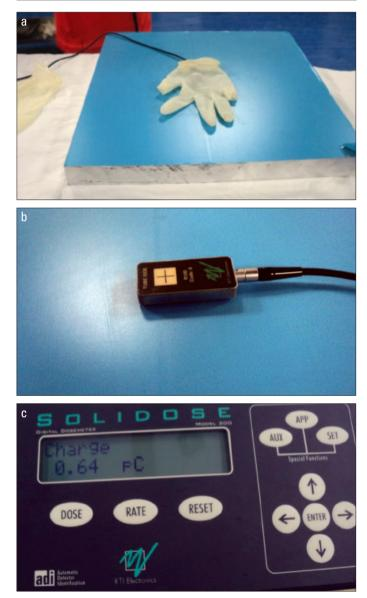
Figure 1 (a-c). An R-100 dose detector was placed into latex gloves at the midpoint of the phantom (a, b). An R-100 dose detector connected to Solidose-300 instant dose-measuring device (c)
