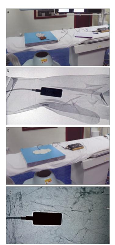
Figure 2 (a-d). Instant dose measurement samples in fluoroscopic device. After the exposure, an X-ray image of the R-100 detector connected to Solidose-300 instant dose-measuring device in lead gloves (a, b). Example of dose measurements of latex gloves coated with CAs and their X-ray image (c, d)
