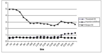
Figure 1. Change in mean threshold values, mean pulse output settings, and mean impedances of lead Accufix II DEC over time
