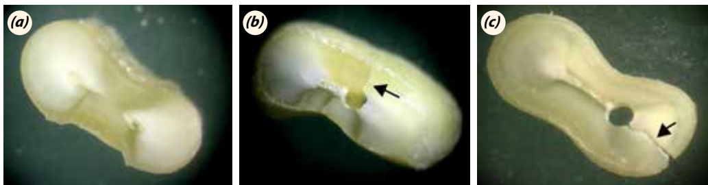
Fig. 1. Examples of microscopic views of samples (a) Section with no defect. (b) Section representing a complete crack. (c) Section representing a complete crack.
