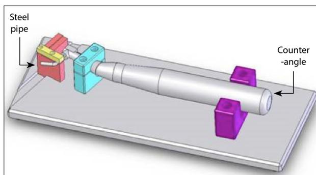
Fig. 1. Fatigue bench diagram.
