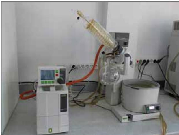
Figure 1. Rotavapor used for preparing liposome formulations
