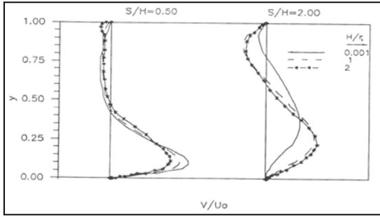
Figure 7. The velocity profile in angular direction (Re = 100, Radial Jet)
