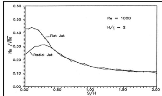
Figure 12. Variation of non - dimensional heat transfer coefficients for flat and radial jets (Re = 1000)
