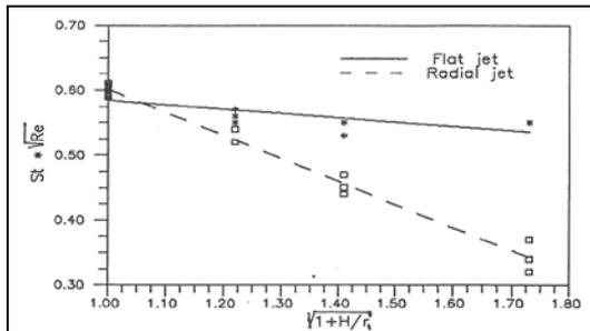
Figure 13. Variation of heat transfer coefficients at stag. Point for flat and radial jets
