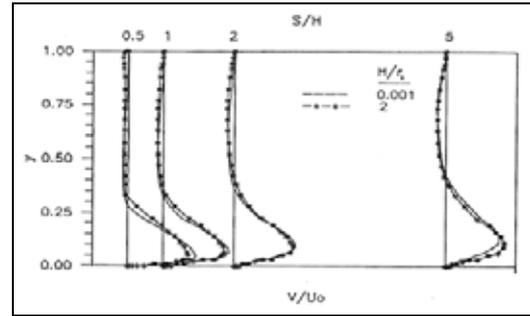
Figure 10. The velocity profile in angular direction (Re = 1000, Flat Jet)
