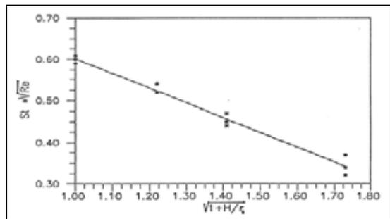
Figure 9. Variation of heat transfer coefficients at stagnation point depending on curvature
