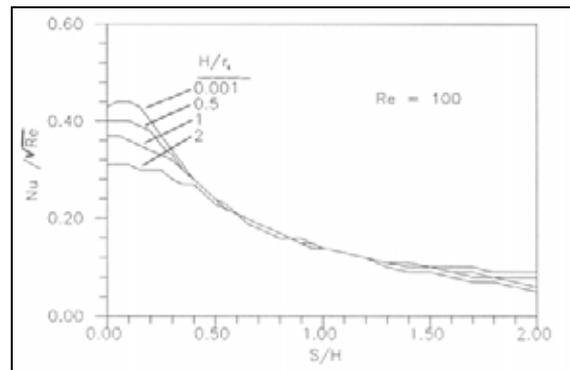
Figure 5. Non-dimensional heat transfer coeff. (Re = 100)
