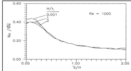
Figure 11. Non- Dimensional heat transfer coefficients (Re = 1000, Flat Jet)
