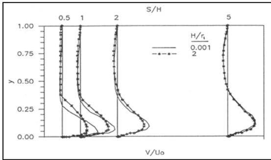
Figure 8. The velocity profile in angular direction (Re = 100, Radial Jet)
