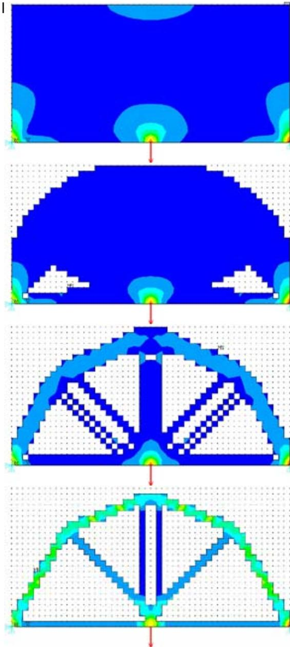
Figure 4. Initial, intermediate and final optimum designs of Example 2.
