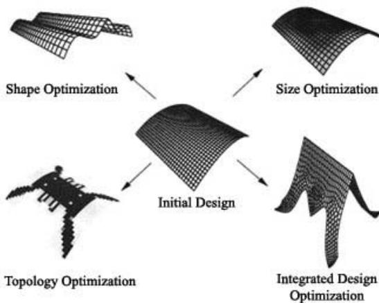
**Figure 1. Various optimization results for a cylindrical shell.**
