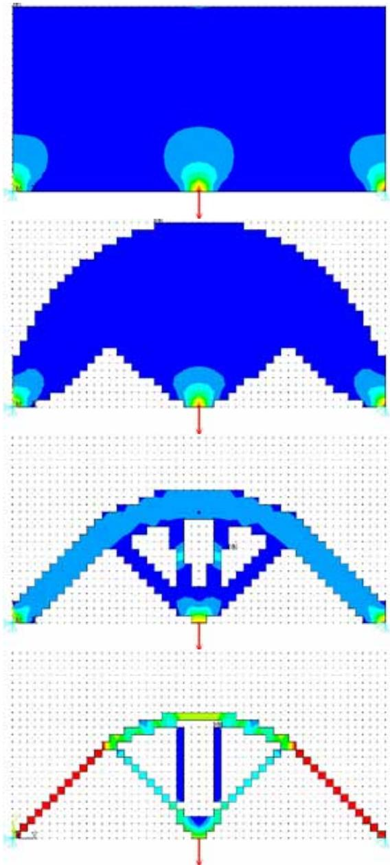
Figure 3. Initial, intermediate and final optimum designs of Example 1.
