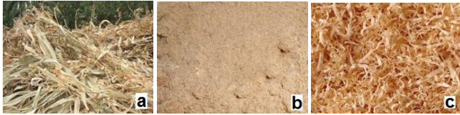
Figure 1: Some natural fibers; corn straw (a), saw dust (b), wood chips (c).
