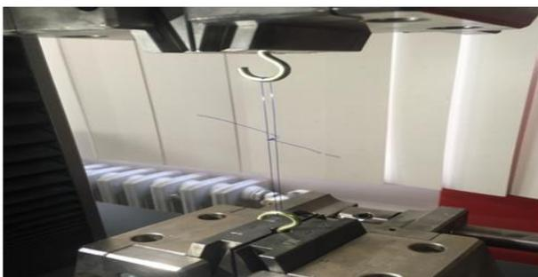
**Figure 1.** Tensile tester (Zwick/ RoellR - Germany) A hook is placed on the pull arms of the device.
