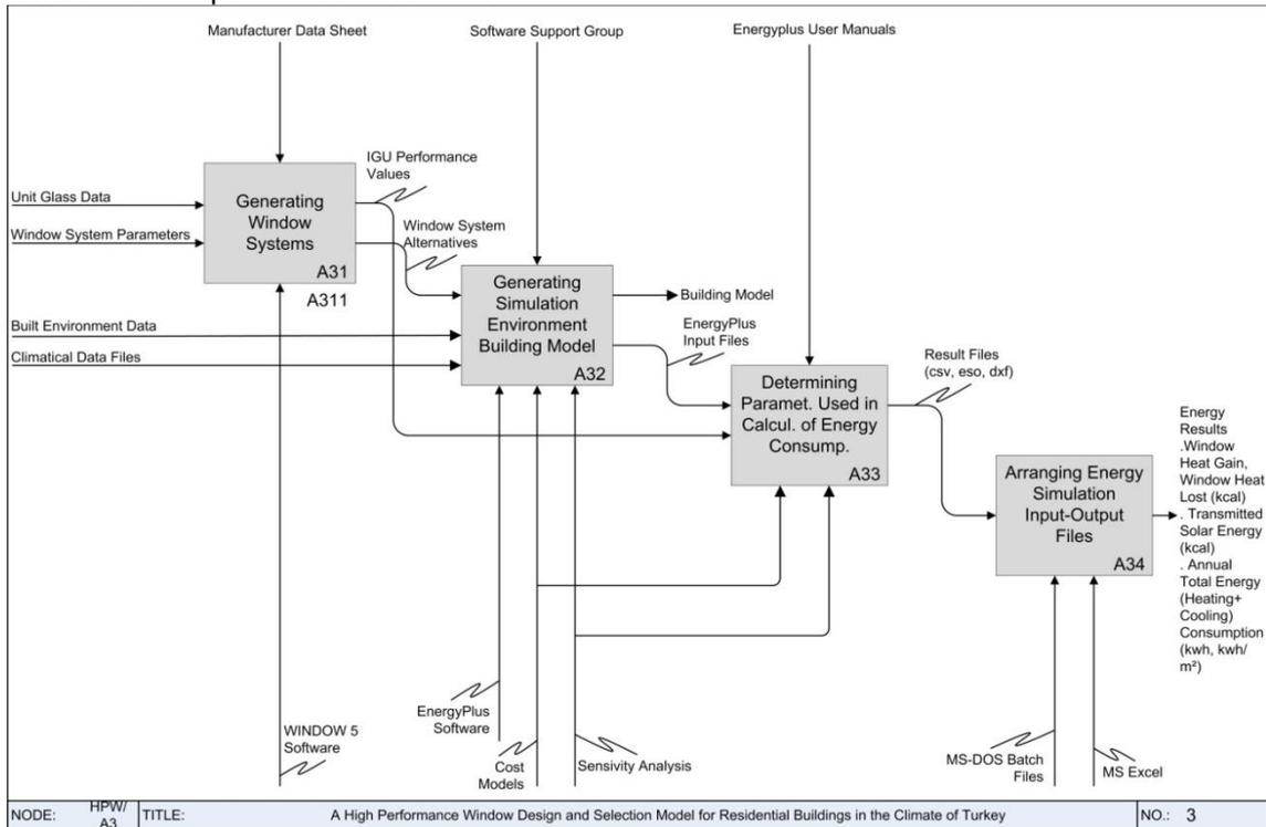
**Figure 3.** The processes of energy simulations with HiPerWin IDEF0 A3 Diagram.
