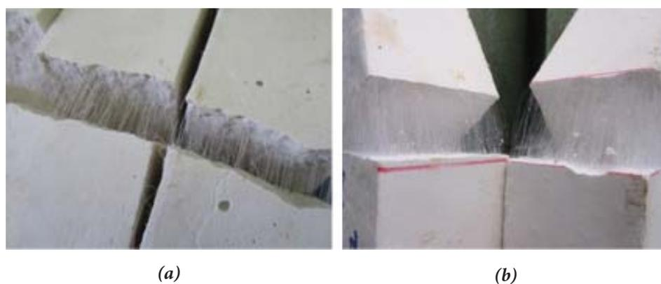
**Figure 1.** rPET fiber-gypsum composite samples.
