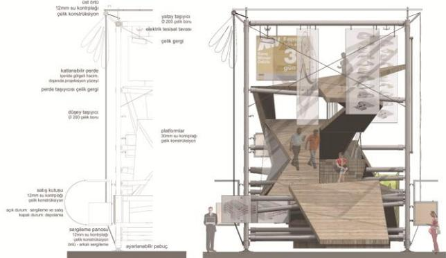
Figure 8. One possible configuration of the System.
