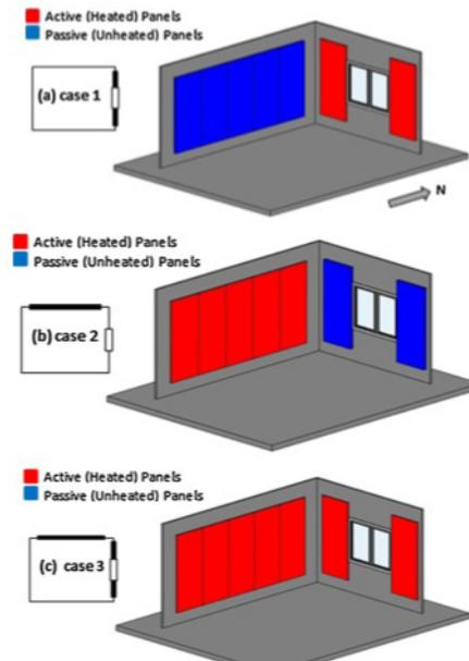
**Figure 5.** Radiant heating wall panel arrangement (TSE 825, 2008).
