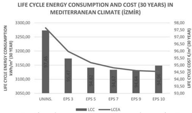
Figure 7. Life cycle energy consumption and cost of EPS with different thicknesses in the Mediterranean climate region (İzmir).
