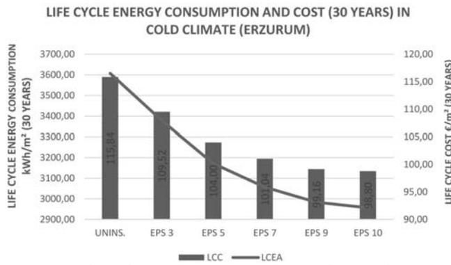
Figure 8. Life cycle energy consumption and cost of EPS with different thicknesses in the cold climate region (Erzurum).
