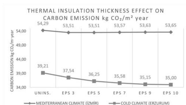
**Figure 4.** The effect of thermal insulation thickness on carbon emissions.
