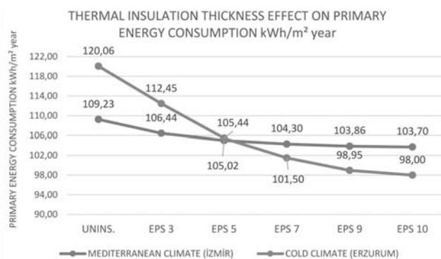
**Figure 3.** The effect of thermal insulation thickness on heating and cooling energy consumption for the case study building.
