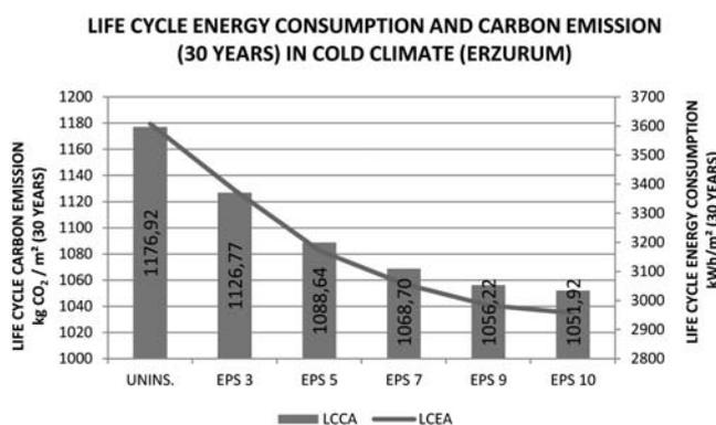
**Figure 6.** The effects of EPS of different thicknesses on life cycle energy consumption and carbon emissions in the cold climate.
