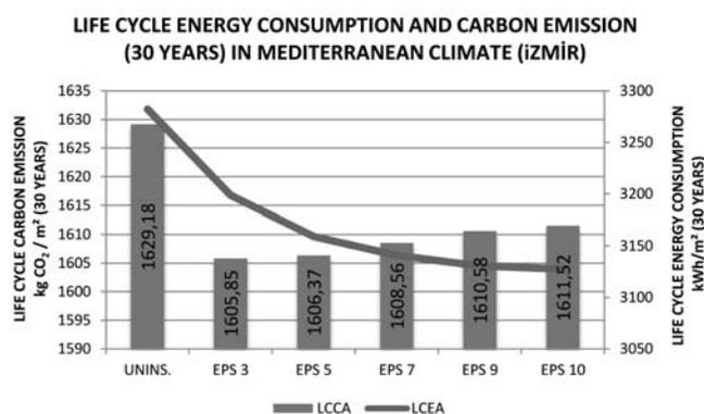
**Figure 5.** The effects of EPS with different thicknesses on life cycle energy consumption and carbon emissions in the Mediterranean climate region.
