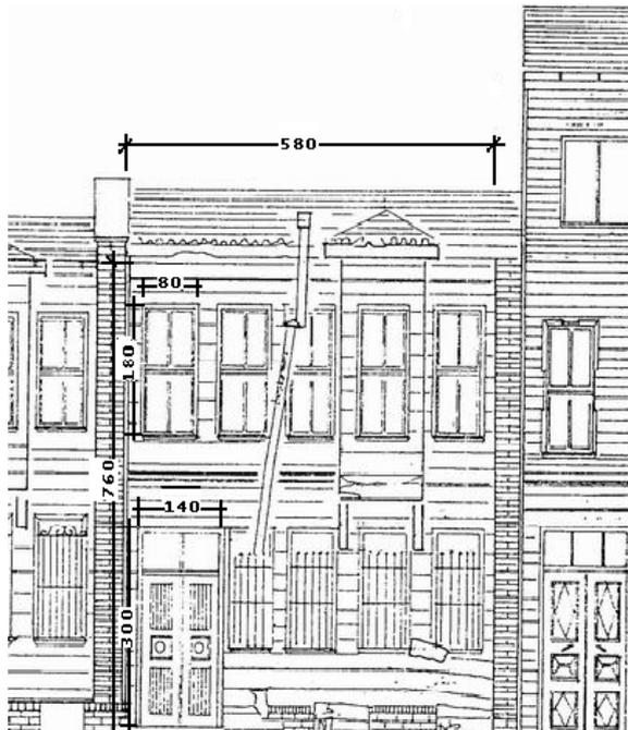
Figure 3. Elevation of the first building
