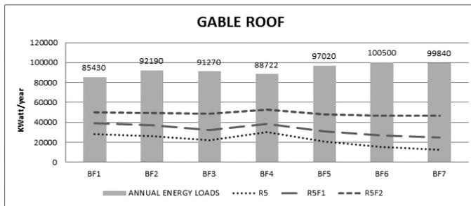
**Figure 4.** Annual energy loads and energy gains with photovoltaic systems in different building forms with gable roof.
