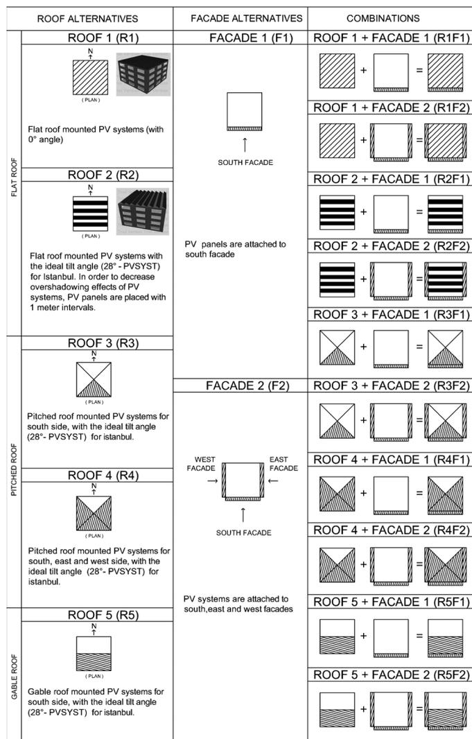
**Figure 1.** Roof and façade combinations for PV system installations.
