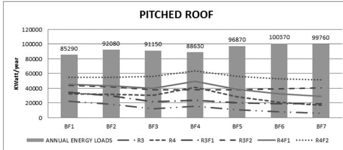
**Figure 3.** Annual energy loads and energy gains with photovoltaic systems in different building forms with pitched roof.
