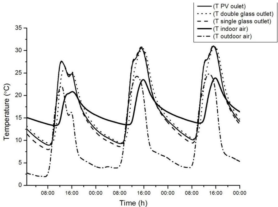
**Figure 7.** The hourly outlet air temperature changes of the PV module, double-glass and single-glass parts.
