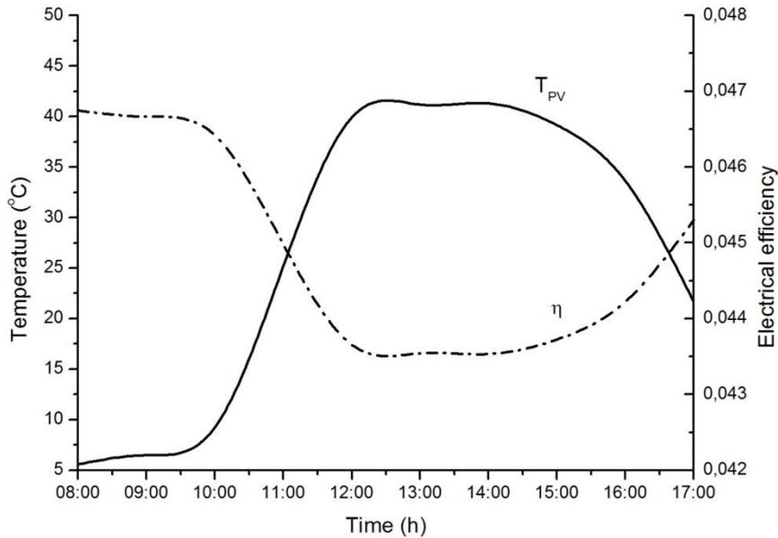
**Figure 9.** The hourly electrical efficiency change with PV cell surface temperature 20 January.
