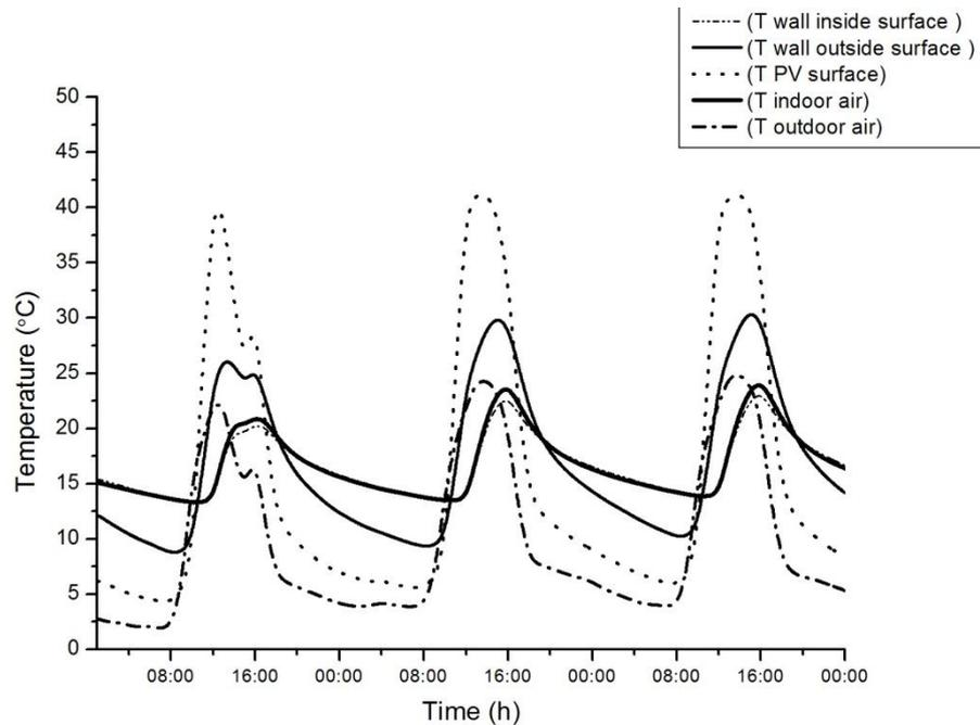
**Figure 8.** The hourly temperature variations of the thermal wall and PV surface.
