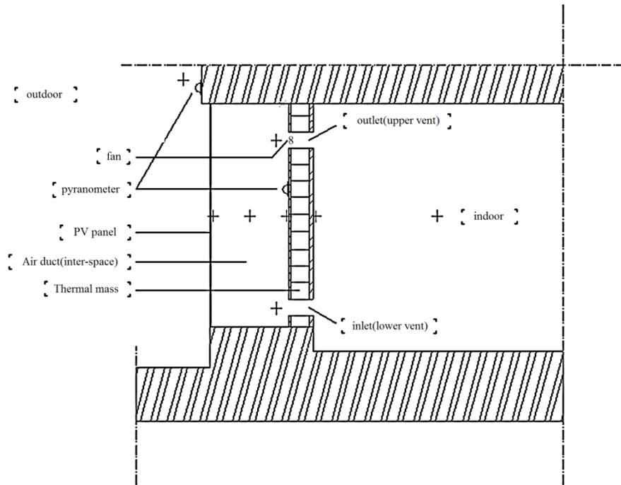
**Figure 2.** Section of the test room when the vents are open for winter heating and the locations of the temperature probes and the pyranometers (Kundakci Koyunbaba, B., Yilmaz, Z., 2012). (+ Temperature testing point)
