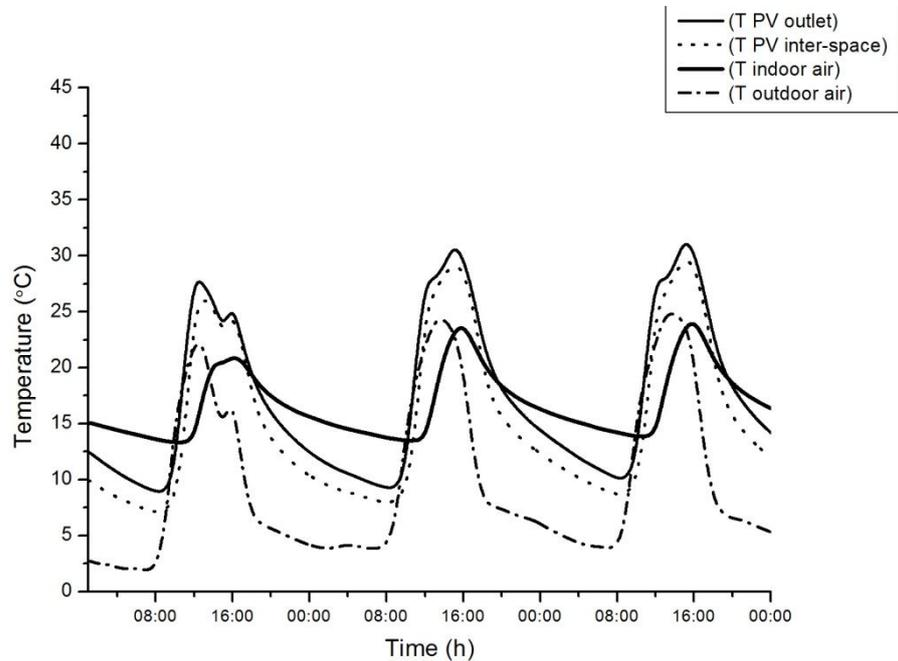
**Figure 4.** The hourly temperature change in the PV module part.
