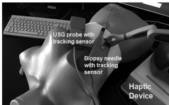
Figure 2. Ultrasound probe and biopsy needle with embedded trackers and the haptic device connected to the biopsy needle.
