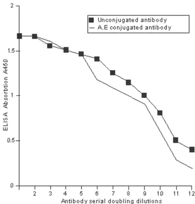
We are reporting here labelling of cTn-I specific 5F4 McAb (9) using an A.E (4-(2-succinimidyl-oxycarbonyl-ethyl) phenyl-10-methyl acridinium-9 carboxylate fluorosulfo-nate). The A.E-conjugated 5F4 McAb was used to develop an immunoassay for *in vitro* detection of cTn-I as a biochemical marker in patients with myocardial damage.
