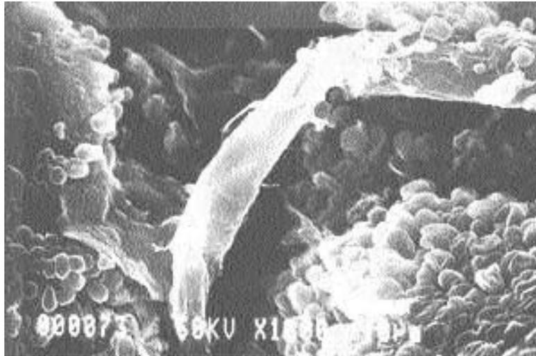
Figure 3: High magnification of spherical globular agglomerates by application of a neutral NaF application.
