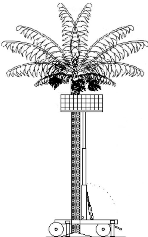
lifts the service platform to the required height via the pulley at the tip of the boom. A modified service platform, shown in Figure 5, is fitted with hand-operated gripper-like clamps to lock itself to the trunk once it is at the desired location.
