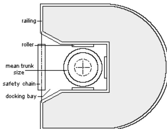
one operator can carry out the hitching-unhitching operations. The design of any trailer, on which the system can be mounted, must allow the positioning of the trailer such that the trunk of the tree is central to the service platform (Figure 1) during servicing.
