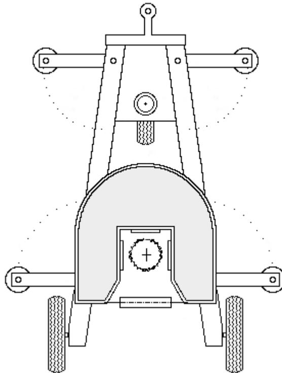
It features anti-slip decking and continuous railing that is one meter high. A docking bay is provided with a tapered opening for facilitating the docking of the platform to the trunk of the tree. The smallest, mean and largest trunk diameters to be handled by the PSS device are marked by circles in Figure 1. The platform is further equipped with rollers around the docking bay for minimizing friction and damage during the raising and lowering operations.
