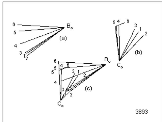
Figure 14: The procedure of synthesis for the second FISC.
