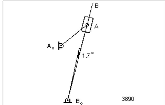
Figure 9: The resulting mechanism for the wiper mechanism.
