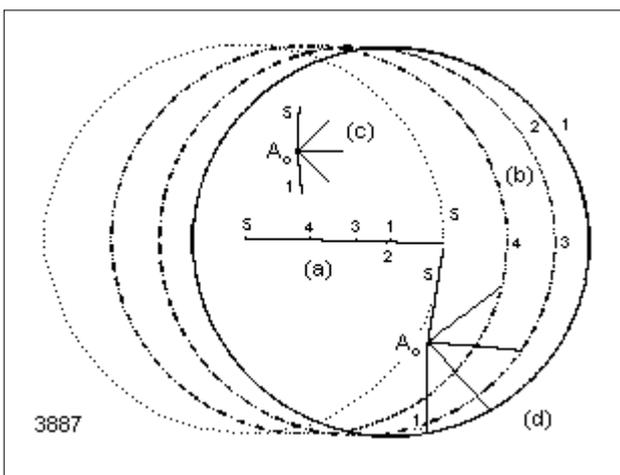
Figure 5: The procedure of synthesis for the slider-crank mechanism.
