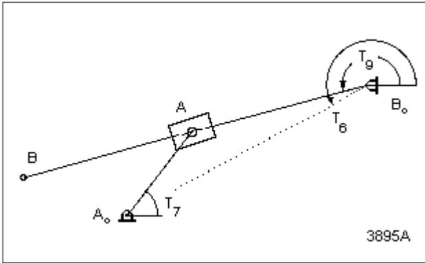
Figure 11: The first FISC of the hack-saw.
