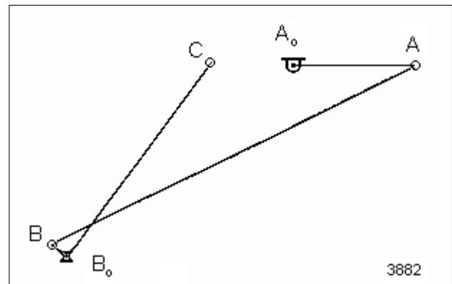
Figure 3: The resulting four-bar linkage.
