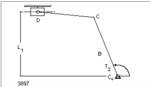
Figure 15: The slider-crank mechanism of the hack-saw.
