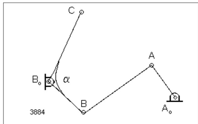
Figure 1: The four-bar linkage to be coordinated.
