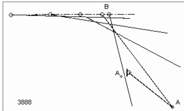
Figure 6: The resulting mechanism for the garage door, with the door at several locations.
