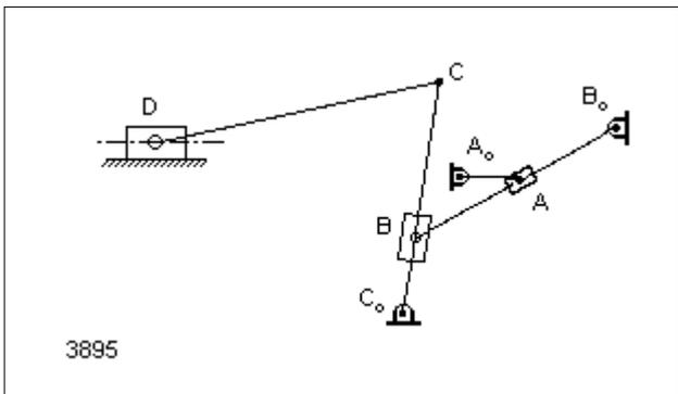
Figure 17: The resulting hack-saw.
