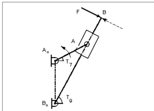
Figure 7: The wiper mechanism.
