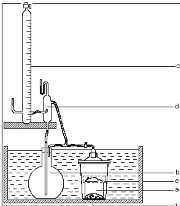
Figure 1: Diagram showing the structure of respirometer: a) glass desiccator-animal chamber; b) oxygen container; c) calibrated burette; d) water type pressure valve with manometer; e) wiremesh cage; f) carbon dioxide absorber (modified from Skvortsov, 1957).
