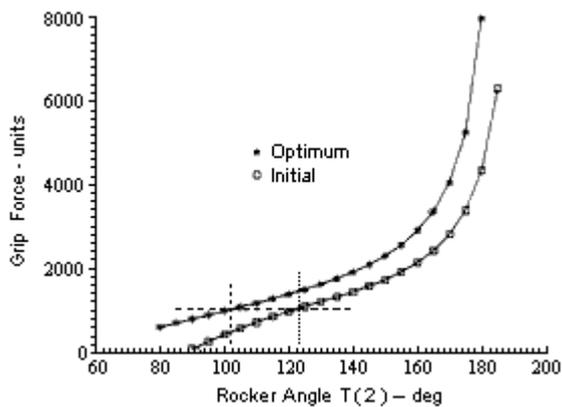
Figure 3: Grip force in the initial and optimized gripper.
