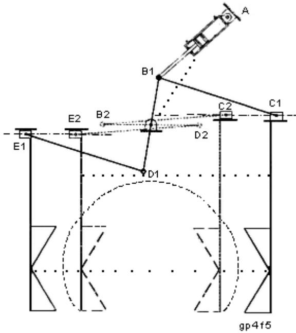
Figure 5: Configuration A for V-notched fingers.
