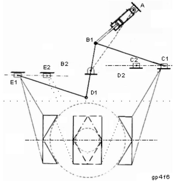
Figure 6: Configuration B for V-notched fingers.
