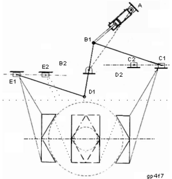
Figure 7: Configuration C for V-notched fingers.
