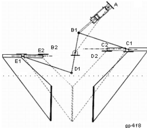
Figure 8: Jaw configuration for flat-faced fingers.
