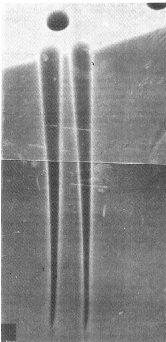
Figure 1: A photomicrograph showing profiles of two long etched tracks along with two etch pits due to energetic uranium ions in a CR-39 (a polycarbonate) plastic track detector. The etched channels are conical in shape and the etch pit openings are uniform in the amorphous matrix of the detector.
