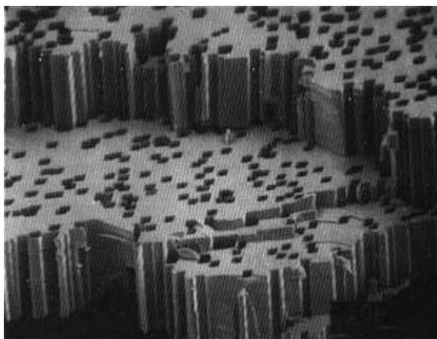
Figure 2: Etched channel profiles and etch pit openings of the etched tracks due to 2380 MeV <sup>84</sup>Kr-ions in the crystalline matrix of a Muscovite mica track detector. The profiles are cylindrical with diamond shaped etch pit openings in the crystalline matrix of mica track detector.
