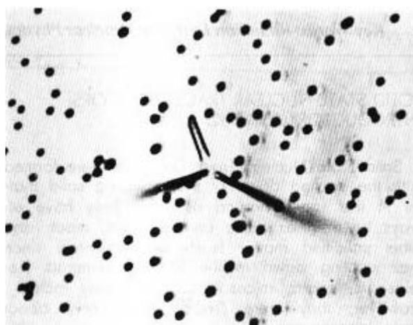
Figure 3: A photomicrograph showing the top view of the etch pits due to energetic <sup>136</sup>Xe-ions in a plastic track detector. A three prong event resulted in the interaction of <sup>136</sup>Xe-ions with a gold target is also present in the photograph.
