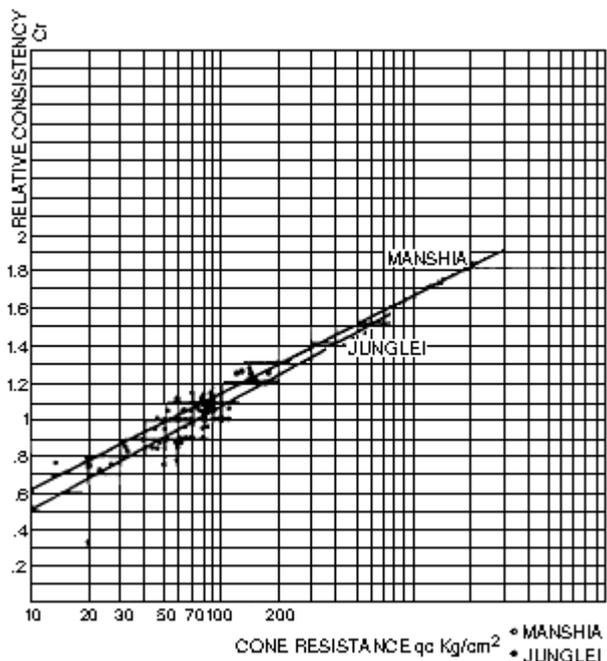
Figure 5: Variation of relative consistency with the cone resistance.
