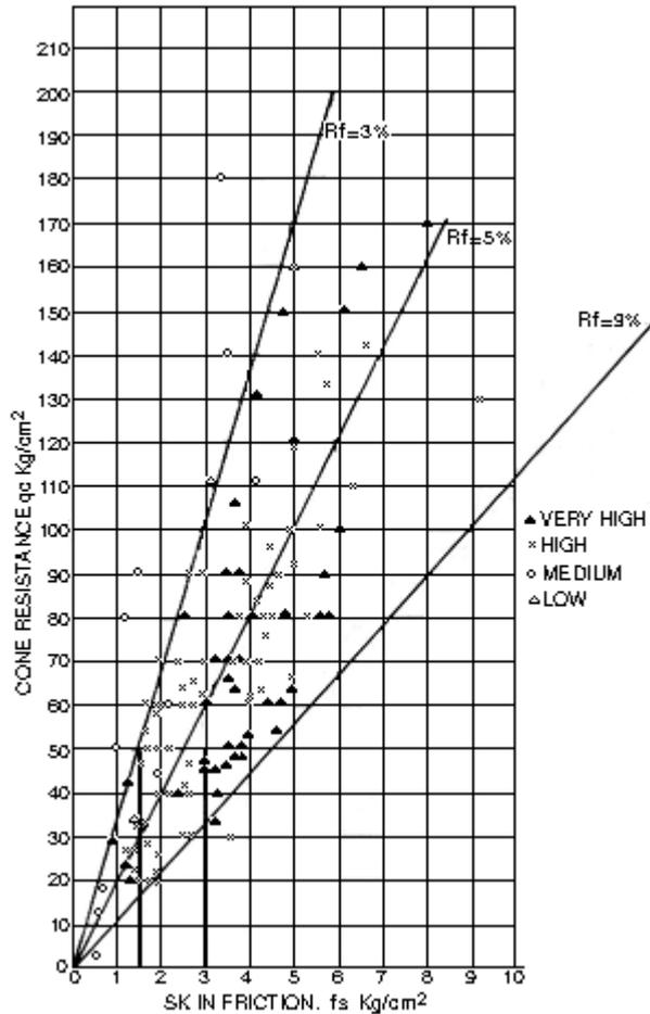
Figure 3: Plot of  $q_c$ ,  $f_s$  with symbols showing the swell potential of the investigated soils.
