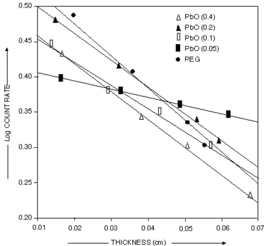
in the probability of interaction between the incident gamma radiation and the shield atoms. This point is further verified from the data (see Table 1) about densities ( $\rho$ ) of these pellets. 2.834 g/cc true density of PEG is enhanced to 3.717 g/cc for the composite containing 40% PbO.
