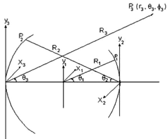
Figure 2: SBFA and coordinate system.
